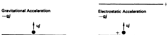
Fig. 2.2 (a) Gravitational acceleration (b) Electrostatic acceleration
